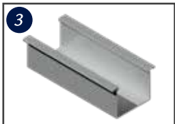
PRIMA Furring Channel 38mm x 28mm x 0.50mm BMT ACC/U/004
