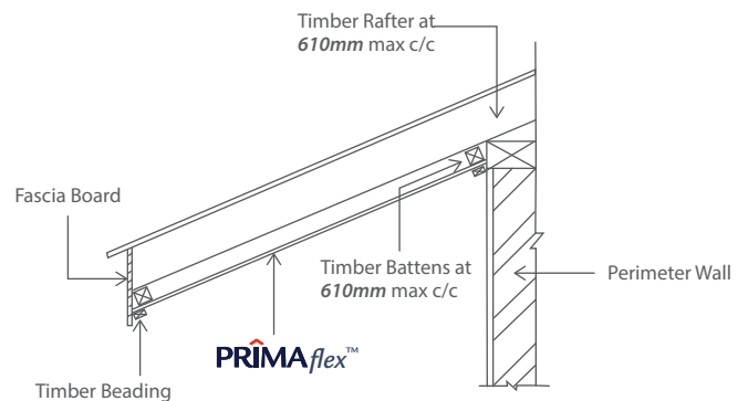
Figure 4.3 – Raked Eaves (for timber structure)
